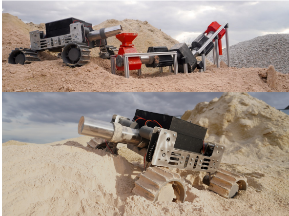
Figure 2: Testing of excavation, transport, and conveyance of fine powders using rover and conveyor.
